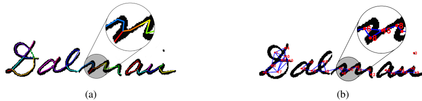
Fig. 18. Construction of the graph representation for a word, (a) convexities from the word vectorization, (b) final grapheme graph.
